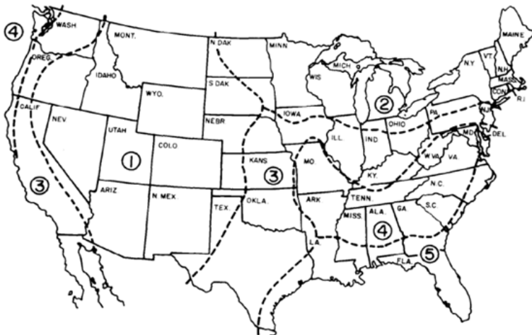
Figure 16: Decay severity zones for wood utility poles (RUS Bulletin 1730B-121).
